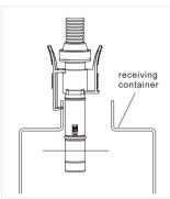
2.Insert fuel gun into receiving container and fixit to the mouth of the container with clip. It isnecessary to make the oil gun and the liquid levelto be 80°~95° as possible.
