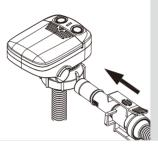
5. Put the fuel gun into the fuel gun placement hole and clamp it with clip.
